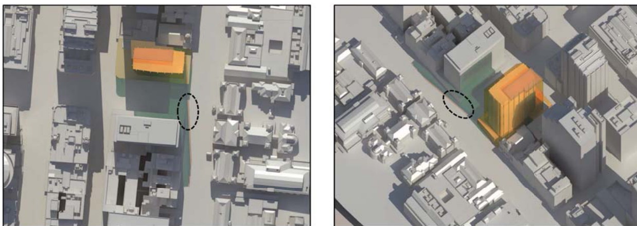
Figure 9: The dashed black line highlights the additional overshadowing on 14 April at 12 noon, which is the orange line at the margin of the overshadowed area, and which falls on Macquarie Street and not on Martin Place.
